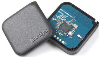
Fig. 2. BLE beacon by WuXi Ghostyu Electronics Company, Ltd. [Online]. Available: http://ghostyu.com .
