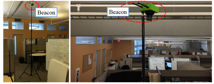
Fig. 2. CMU localization dataset [33] consists of the beacon data collected from ten beacons mounted on different tripods.
