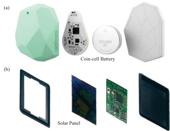
Fig. 1: There are two common types of beacon in the market: (a) battery-powered beacon, and (b) solar-powered beacon.
